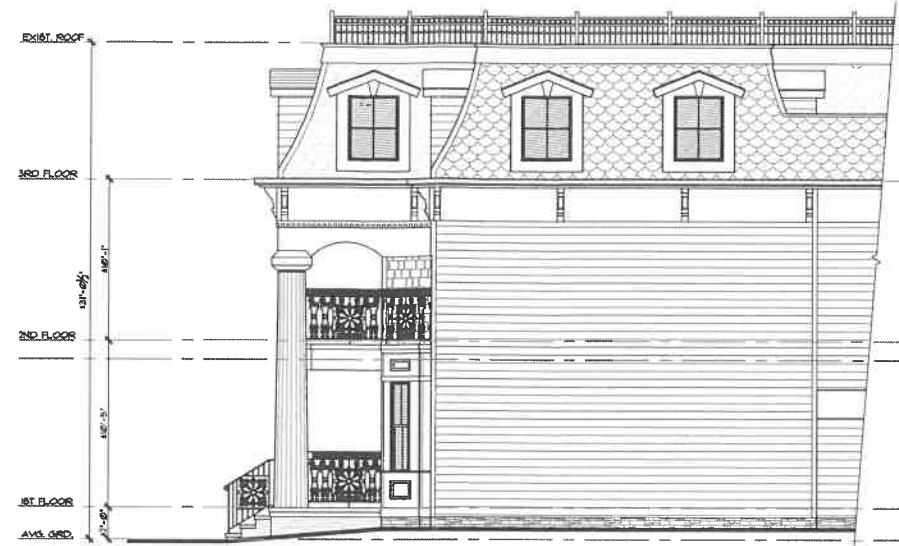
2 EXISTING PARTIAL SIDE ELEVATION (EAST) SCALE: 3/16"=1'-0"
