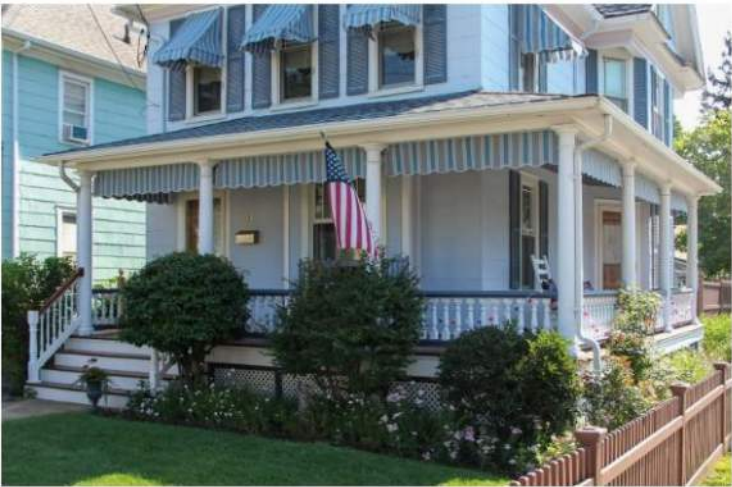
Broad wraparound porch with turned columns, balustrade, skirting lattice, and striped fabric awnings.
